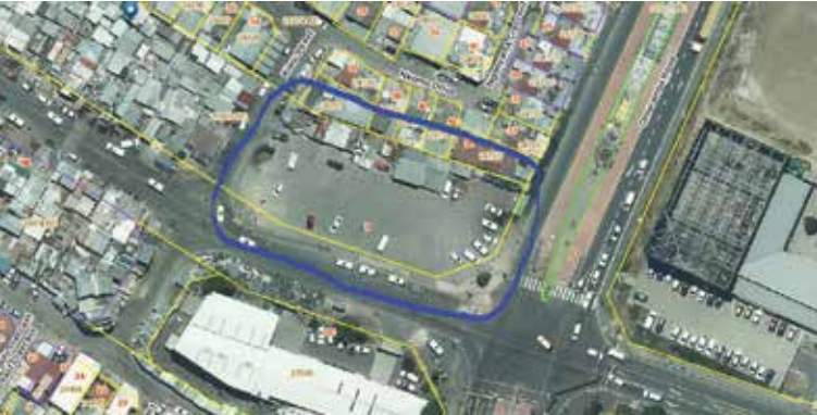
Improved interchange on the way: The upgrade to the Joe Slovo public transport interchange (PTI) in Milnerton (circled in blue above) is in full swing and should be completed by February 2026. Taxi operations have temporarily relocated to the corner of Freedom and Democracy ways. Work includes the surfacing of the current unsurfaced area, improvements to a section of the existing road leading to the PTI, and the construction of sidewalks and sewer and stormwater systems (including kerbs, channels, manholes and catchpits). New road signage and road markings will also be installed.
